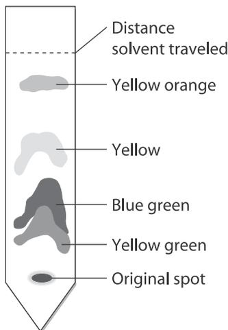
Several drops of concentrated green pigment extract obtained from spinach leaves were placed near the bottom of a strip of highly absorbent paper. When the extract dried, the paper was suspended in a test tube containing solvent so that only the tip of the paper was in the solvent. As the solvent was absorbed and moved up the paper, the various pigments within the extract became visible, as shown in the diagram.
