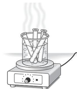
**Figure 9-22. Hot water bath:** A hot water bath is used to heat test tubes that contain a flammable liquid such as alcohol.
