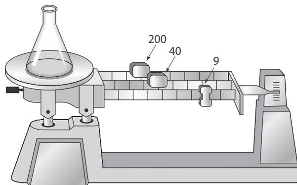
With the riders in the positions indicated, what is the mass of the object on the pan of the balance?
