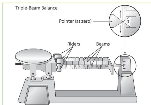
**Figure 9-6. Triple-beam balance**
